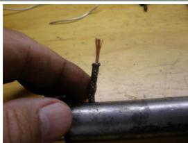
Prepare the wire to be soldered by cutting away about 1/4in of insulation. Place the wire over the bushing, and cut about 1/4 in below the bottom of the bushing. Then strip the wire and prepare for soldering.
