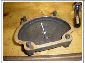
The housing plate screw will allow the sector shaft to move back to a certain point in the housing. If you adjust this to far in, the shaft will become to tight, if it is to loose, the teeth may skip in the worm gear. Note: here you are preparing to install the copper washers. It is a good idea, to heat red hot, and cool in water, the copper is annealed and all previous stresses from tightening are relieved
