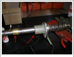
\*check\* make sure you have your top CUP and HOUSING TOP COVER (and shims) prior to soldering... make it a lot easier for fitting. Add Flux to surface area and wire prior to soldering otherwise solder will not stick. Place wire on copper bushing and solder on top of wire until it melts to bushing
