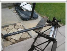
This steering was removed from a 1944 gpw. From the start we see the steering tub is bent, and by the looks of it, most likely will need some replacement parts.
