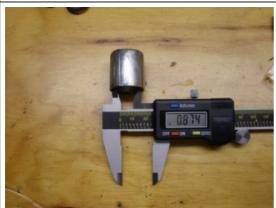
Measuring the inside diameter of the bushings will help you see how much the diameter will decrease when pressed in.
