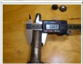
Last, measure the shaft as well. This should be within a .001 value to the inside diameter of the bushings.
