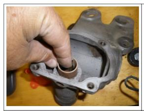
Once the bushings broke down a bit, they were easy to pull right out.
