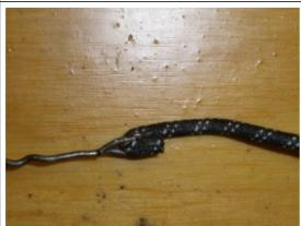
The hole your going to pull through in the shaft is just barely bigger than the wire, so this will be very tight when you pull it through. Here, you see to hook a very small piece of horn wire to your pull wire.
