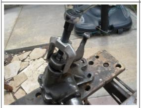
With an inexpensive puller, we pull the arm off. Note: don't try pounding this off as it will require a puller to do it correctly without damaging the arm.
