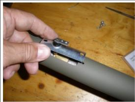
Now install the brush on the contact tube. Place the tube down the shaft and over the housing fitting, down as far as it will go and tighten up.
