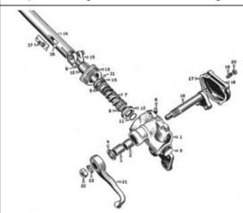
The Steering component in a WWII jeep is not very complicated. But, almost all restore projects have very old, probably rusting steering components that need to be looked at before you can drive safely. Here you see a breakdown of the steering box components from the TM-10-1513
