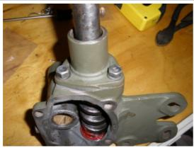
Now install your main shaft cover tightening the bolts down. When tightened, turn the main shaft and tug up and down. If you have play up and down, then you need to take a shim out, if turning is really tight, then add a shiim. In this case, it was a little loose with play in the top and bottom.
