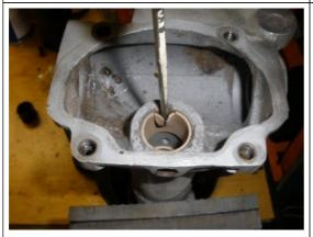
\*back to the housing\*. Now let's remove the housing bushings. The TM's mention to use a chisel to pop the bushings out. In this case the copper bushings were very brittle and crumbled almost immediately upon impact.
