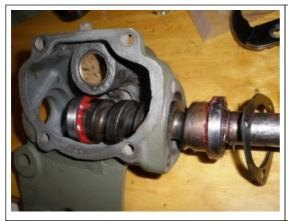
Run your shims up on the main shaft, and push your worm gear into the housing. It should be a little snug, but will fall into the housing by a firm press into position.
