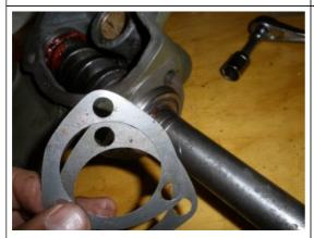
In this case, I needed to reduce the shims down to two (from three) to get a snug fit. It was about .018 measurement. Repeat the steps to put back on and test. Ahh, much better. Turns well with no play.
