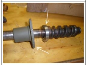
After we clean the shaft and it's worm gear, we will prepare to install the new cup, housing cover, and the contact bushing. First, install the cup on the shaft with the cup to hold the ball bearings toward the gears. The next step will be to install the contact bushing which requires some pounding, therefore, temporarily tape the cup at the bottom of the shaft near the gear.
