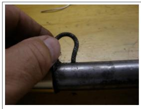
You want to pull the excess wire through with just a little extra at the top of the shaft. If you don't, you will have some back pressure from the wire when you try and apply the nut.
