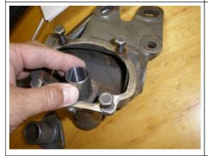
Next, line up the bushings to be pressed in. Here you see the bushing with the grove all the way to the end which will feed the lubrication to the shaft. You will want to line up the other bushing and press through the other side.
