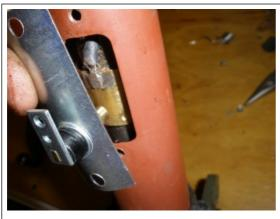
Here you see the contact will run on the bushing for the horn just fine. It lined up well and will not hit the soldering.
