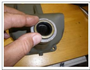
Here, install the housing seal by tapping it into the housing. It should be good and snug.
