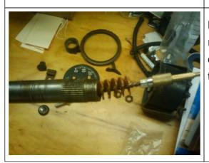
Next, check the inside of the shaft for rust. Here I used a 20 gauge gun cleaning brush and rod to clear out all the rust from the shaft.
