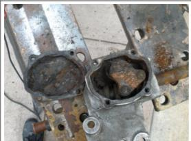
Now unscrew the 4 bolts on the side cover. With the side cover off inspect the inside of the steering housing. Here you can see there was not much maintenance done on this.
