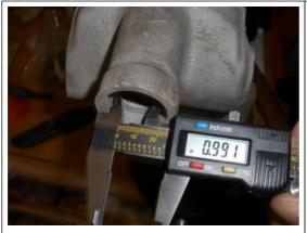
Prior to installing your replacement bushings, measure the inside diameter of the housing, and the outside diameter of the bushings. The bushings should fit tight, but the tighter they are, the smaller the inside diameter of the bushings will become when pressed in.
