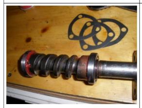
The retainer ring on the upper side is a bear! You have to try and get it around the shaft and in its location without bending it all up. Here it was pressed around the shaft and placed into its location.
