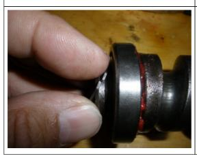
Press one side of the ring around the ridge on the worm gear and press the ring around the ridge and it will snap into place. This side is the easier of the two.
