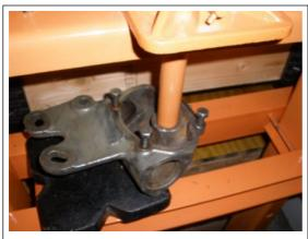
Next, press the bushings into the housing. You should line up the grove on the bushings so that the lubrication will flow to the shaft
